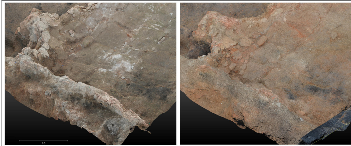
Figure 5: Left - surface created out of data from 2006, right - segment of point cloud used for comparison
