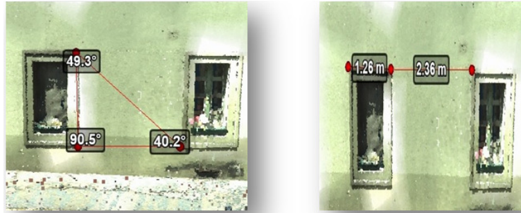
Figure 4. Measurements on merged point cloud
